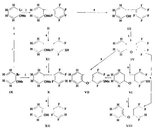
Reagents: 1, Li in Et<sub>2</sub>O; 2, C<sub>6</sub>F<sub>6</sub> in Et<sub>2</sub>O; 3, 4H-C<sub>6</sub>F<sub>4</sub>Br/Cu; 4, AlCl<sub>3</sub>; 5, K<sub>2</sub>CO<sub>3</sub>, D.M.F.; 6, NaSH, D.M.F.; 7, Ni; 8, McSNa/McOH; 9, LiAlH<sub>4</sub> in Et<sub>2</sub>O; 10, CH<sub>2</sub>N<sub>2</sub>.
